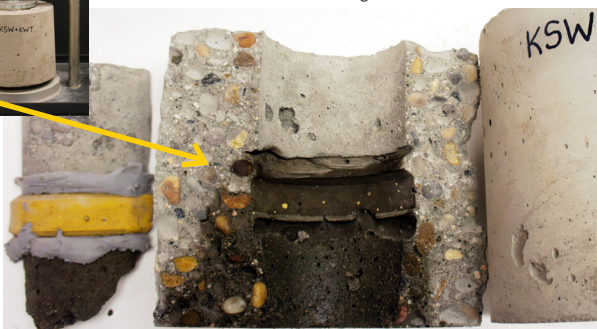
Proven 0.8 MPa (8 bar) water stopping performance in modified DIN 1048-5 testing
