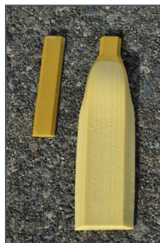
Before and after water exposure
